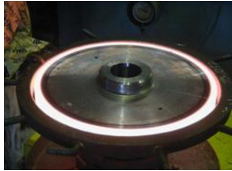
One time quenching of all gear teeth
