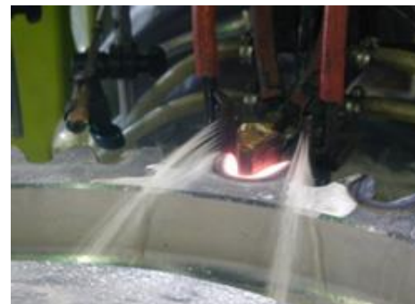
One-by one quenching of gear tooth
