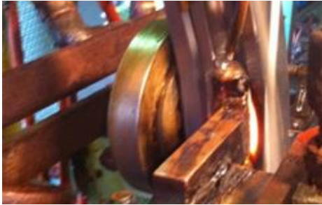
Groove surface zone quenching
