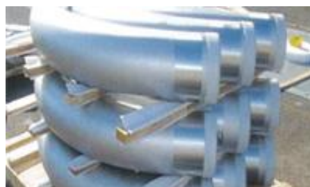
Bends for pneumatic piping
