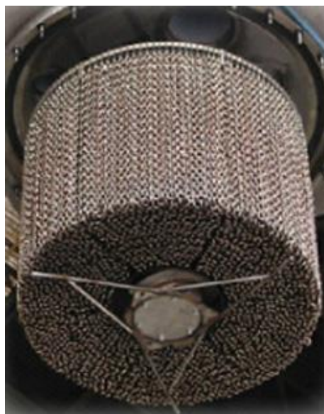
Heating structure for superheating
